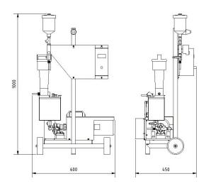
Due to volatility of the solvents, a change in the viscosity of your printing ink is inevitable. Our viscosity control device monitors the ink and automatically dispenses solvent as required to maintain consistent ink viscosity levels. The result is a uniform print of the highest quality. We recommend this viscosity control device for all applications where solvents tend to evaporate quickly and for line speeds greater than 500 m/min. (1640 fpm)
